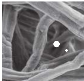
Enlarged top views of media (at the same magnification) White circles represent the diameter of a 2µ and a 5µ particle.
