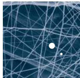
Enlarged top views of media (at the same magnification) White circles represent the diameter of a 2µ and a 5µ particle.
